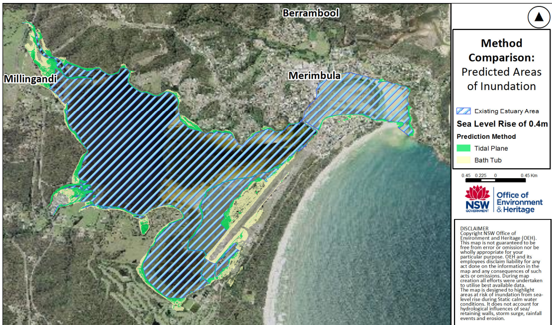
Figure 7. Plot showing example of comparison between predicted inundation using tidal plane and bath-tub methods.
